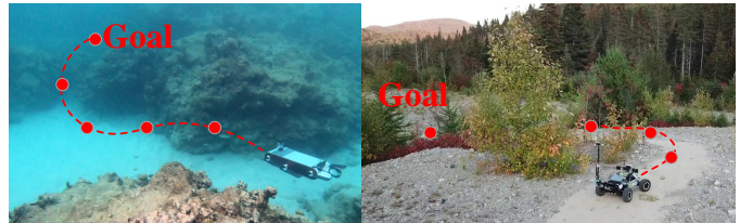
Fig. 1. Navigation example for both an underwater and ground vehicle. Examples of waypoints to be visited are illustrated by the red circles (although in practice they are usually much more widely separated). The actual trajectory used to achieve them in the presence of obstacles is at the discretion of the learned policy.
