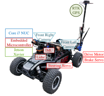
Fig. 3. Off-road vehicle used for real-world experiments. In practice, only one forward-facing camera is used in this work.
