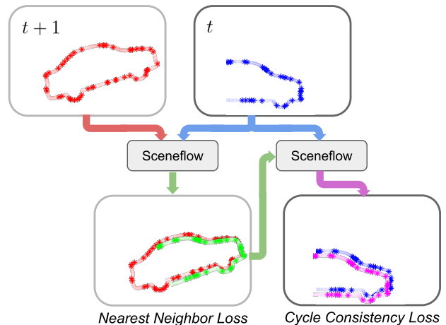
Fig. 1: We use two self-supervised losses to learn scene flow on large unlabeled datasets. The “nearest neighbor loss” penalizes the distance between the predicted point cloud (green) and each predicted point’s nearest neighbor in the second point cloud (red). To avoid degenerate solutions, we also estimate the flow between these predicted points (green) in the reverse direction back to the original point cloud (blue) to form a cycle. The new predicted points from the cycle (purple) should align with the original points (blue); the distance between these two set of points forms our second self-supervised loss: “cycle consistency.”
